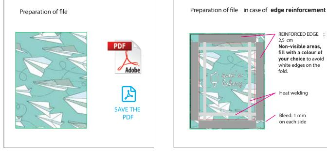
REINFORCED EDGE : 2,5 cm Non-visible areas, fill with a colour of your choice to avoid white edges on the fold. Heat welding
